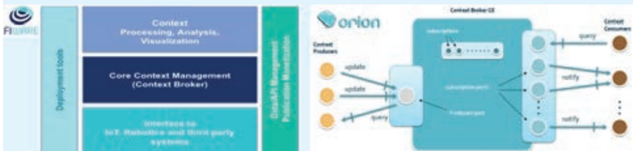
Figure 4-8 ORION context broker generic enabler. Source: FIWARE
